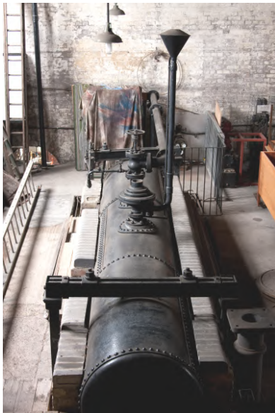
Haythorne Davey steam pumping engine
